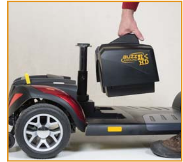
Step 2: Pull out the battery pack!
