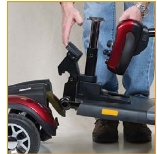
Step 4: Pull forward on the drivetrain release lever to separate the front and rear frame sections!
